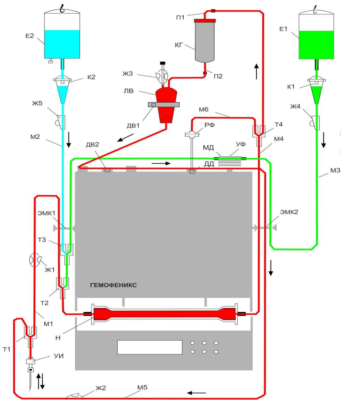
**Fig.1. Extracorporeal circuit diagram hemofiltration "Hemofenix" device.**
